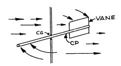
This drawing shows a vane added to one end. This moves the CP away from the CG. The force of the flowing air on the vane causes the object to point into the flow with the CP behind the CG. Ordinary finned rockets use this form of stabilization. Fins are like feathers on an arrow. They put the CP behind the CG.
