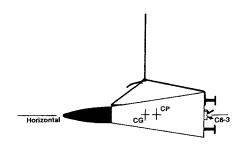
Adjust the position of the knot so the Space Clipper™ hangs horizontally. This balances the model at its CG. The CG should be at the second payload bay hinge mark on the AeroShroud™. Use a bit of tape on the base to secure the string in position.
