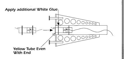
IMPORTANT: Test fit the Aeroshroud first before applying any glue.
