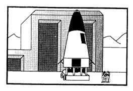
spaceship will be towed to the maintenance hangar. Otherwise, the ground crew pumps propellants — liquid hydrogen and liquid oxygen — into the spaceship. Passengers go aboard or palletized cargo is loaded. And the Delta Clipper is on its way again in less than a day.
