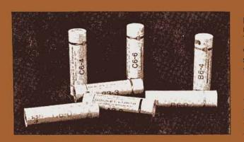
The AVI Thruster-18® model rocket motors are miniature solid propellant rocket units specifically designed for propelling the AVI model rockets. They are made in a range from Type A through Type C. They are the USA "standard" size of 18 millimeters diameter (0,690 inches) and 70 millimeters long (2,75 inches). This standard 18 x 70mm, size will fit most model rockets and may therefore be used to propel models other than the AVI kits.
