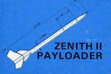
Big. easy-to-build 2-stager to introduce you to multi-staging. Transparent payload compartment 0.945" dia. x 3.15" long capable of lifting 2 oz. to more than 1000 feet. Basic diameter 0.945". Length 22-7/8". Basic weight (no motors or payload) 1.60 oz. Recommended motors: C6-0 or B6-0 in booster, A3-4, B6-6, or C6-6 in upper stage.
