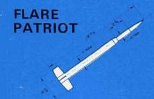
NAR Quadrathon model—parachute duration, altitude, payload carrying, and spot landing. Payload compartment 0.748" dia. x 1.89" long takes up to 2 oz. Booster body 0.984" dia. 14" poly recovery chute. Basic weight (no motor or payload) 1.06 oz. Recommended motors: A3-2, B3-3, B6-4, C6-4.
