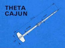
Patterned after NASA rocketsondes. Mini-payload compartment capable of taking payloads up to 2 oz. in space 0.55" dia. x 7.00" long. Basic booster dia. 0.788". Length 21" overall. Basic weight (no motor or payload): 0.95 oz. 10" poly recovery chute. Recommended motors: A3-2, B3-3, B6-4, or C6-6.
