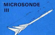
This one is NOT for beginners! 3-stages to loft payloads to altitudes of more than 1000 feet. Parachute recovery of top stage; tumble recovery of booster stages. Maximum payload capability 1 oz. in 0.945" dia. x 3.15" long. Booster dia. 0.788". Length 24.75". Basic weight: (no motors or payload): 1.6 oz. Recommended motors: 1st stage C6-0 ONLY — 2nd stage C6-0 or B6-0 — top stage A3-4, B6-6, or C6-6.
