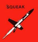
The Miniroc for the brute-force types who enjoy cloud-bursting. The smallest airframe that could be put around a Minijet and safe streamer recovery. Real low-drag design. 3-caliber ellipsoidal balsa nose. Sheet balsa fins are special high aspect ration low-drag shapes.
