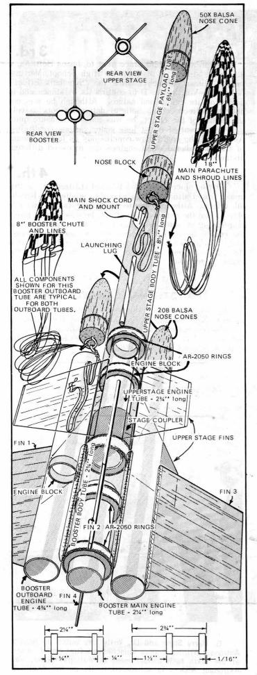
6. Glue the two 4-3/4" long pieces of BT-20D to the booster body tube. The ends of the side tubes should be even with the end of the engine mount tube. Check to be sure all three tubes are aligned perfectly, then set the unit aside to dry.
