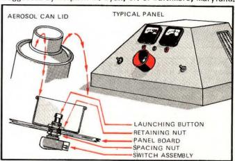
When mounting the launch button (such as the SWM-1 switch) also drill a  $1/2^{\prime\prime}$  hole centered in the top of an aerosol can lid as you drill the 1/2" hole in the panel. Install the switch shaft through the panel from the underside, invert the cap and install it over the switch shaft followed by the retaining nut as shown. Thus protected, your launching button is less likely to be accidentally pressed prior to reaching the end of a countdown.
