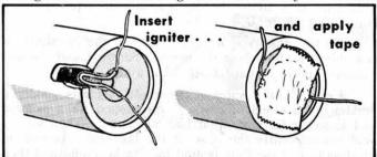
then, instead of tamping wadding in, they spread the leads and apply a square of masking tape to the nozzle and leads as shown. The eraser on the end of a pencil is good for pressing the tape securely into place.
