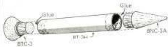
2. Apply glue just inside the other end of the escape motor tube and slip the tail cone into place as shown in Fig. 1.
