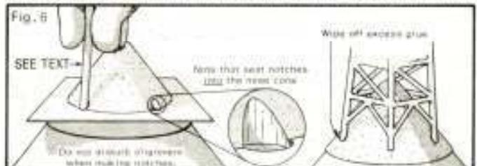
dowel or a 1/16" drill bit. Apply a drop of glue to each notch and fit the base legs of the tower structure into place. Wipe off any excess glue and let the assembly dry completely.
