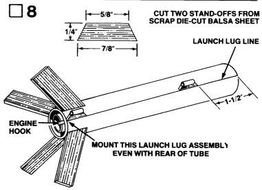
Cut two launch lug stand-offs from the remaining scrap of the die-cut fin sheet, to the dimensions shown. Use a sharp modeling knife to cut the launch lug (part F) into two 5/8" long sections. Glue the two launch lugs to the two balsa stand-offs, align them straight, and allow to dry. Now glue the two launch lug assemblies on the launch lug alignment line in the positions shown. Be sure these are mounted straight on the tube before the glue sets.
