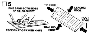
Fine-sand the balsa sheets (part E), then carefully remove the die-cut fins from the sheet. Free the edges with a sharp knife. Sand the leading, tip, and trailing edges of the fins round. Leave the root edge square. Do not discard the remaining balsa sheet just yet.
