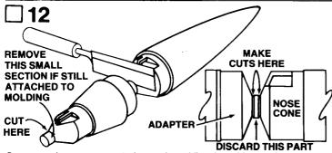
Separate the nose cone/adapter (part H) using either a sharp modeling knife or modeler's saw. Use the grooves molded into the part as cutting guides. Discard the small section of plastic removed between the two parts as it is not used. You will also need to cut away and discard the small tubular section at the base of the adapter if it has not already been removed.
