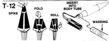
Hold the parachute at its center and pass the other hand down it to form a "spike" shape. Fold this spike in half. Roll parachute into tube shape to fit easily into body. Pack 'chute into the tube on top of the wadding. Pack the shroud lines and shock cord in on top of the parachute and slip the adapter section into place.
