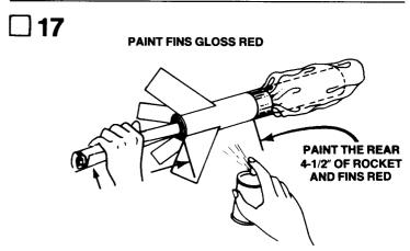
Apply masking tape and paper to cover and protect the areas which will remain white (See the panel or Decor Layout illustration.) Paint the fins and the rear of the body tube red. Carefully remove the masking tape and paper as soon as the paint is dry.
