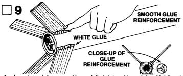
Apply a glue reinforcement to each fin joint and launch lug. Holding the model level, apply a line of glue to both sides of each joint. Smooth out the glue with your finger. Keep the model level until the glue dries.
