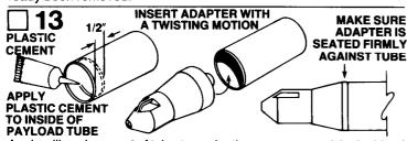
Apply a liberal amount of tube-type plastic cement around the inside of one end of the payload tube (part I). The cement should be about 1/2" from the end of the tube. Insert the adapter with a twisting motion and its shoulder is seated firmly against the payload tube end. Set aside to dry thoroughly. Cement the nose cone into the payload tube, in exactly the same manner as the adapter. Set aside to dry thoroughly.
