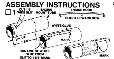
Mark the engine mount tube (part A) 1/4" and 1-5/8" from one end. Use a sharp modeling knife to cut a 1/8" wide slit at the 1/4" mark. Insert one end of the engine hook (part B) into the slit and lay the hook into the glue straight along the tube. Wrap two layers of masking tape around the hook and tube with one edge of the tape next to the mark as shown.
