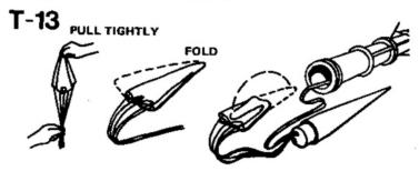
Gather the parachute as shown, then fold into a triangular shape. Fold again and insert into rocket body.
