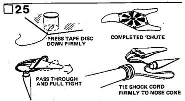
Cut out the parachute (part Q) on its edge lines. Cut three 24" lengths of shroud line (part R). Attach line ends to the top (printed side) of the parachute with tape discs (part S) as shown. Pass the shroud line loops through the nose cone eyelet. Pass the parachute through the loop ends and pull the lines tight against the eyelet. Tie the free end of the shock cord to the eyelet with a double knot. Pack 'chute and shock cord into rocket body. Slide nose cone into place.
