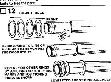
Apply a thin line of glue around the body tube at the fourth tube line from the front and on the front ends of the wood strips. Slide one of the 12 rings down the body tube onto the line of glue and against the wood strips. Then apply another thin line of glue around the body tube at the third tube line from the front. Slide another ring in place on this tube line. Repeat adding rings for number 2 and number 1 tube lines.
