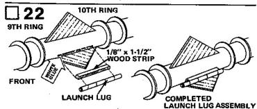
Locate the 1/8" x 1-1/2" long square wood strip left from step 9. Glue strip to tube and fin side of one of the triangular fins centered between the 9th and 10th rings as shown. Then glue launch lug (part P) to the top of the strip so it is centered on the strip and fin.
