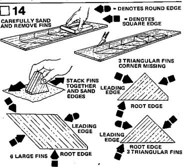
Fine-sand both sides of the balsa fin sheet (part L). Carefully remove the fins from the sheet. Use a sharp knife to cut free the corners and edges. Stack the six large fins, the three triangular fins, and the three triangular fins with one corner missing as shown. Sand all edges smooth and straight. Sand round the leading edges only. The root edges (body edges) must be square. Be sure to sand the three triangular fins with the corner missing to shape shown on the kit pattern sheet.
