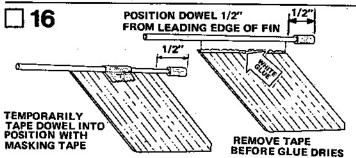
Glue a dowel to each of the 6 large fins as shown on the pattern sheet. The launch lug end of each dowel should project 1/2" forward from the leading edge of each fin. Temporarily tape each dowel in position with a short strip of masking tape until glue dries. Remove tape as soon as glue has set. DO NOT wait till the glue is completely dry.
