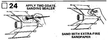
When all glue on the outside of the model is dry, prepare the balsa fins for painting. Apply at least two coats of sanding sealer to the fins and wood strips. Let dry and sand lightly with extra-fine sand-paper between coats. Do this until the tiny grain lines in the wood are filled and everything looks and feels smooth.
