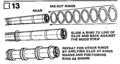
After glue has "set" on the first four rings, turn rocket body around so the rear of the body is in your right hand. Apply a thin line of glue around the body tube at the tube line ends of the wood strips. Apply glue to the ends of the wood strips. Slide a ring down the tube onto the glue and against the wood strips. Repeat, applying glue on the tube lines and positioning all the remaining rings. Set the assembly aside to dry.
