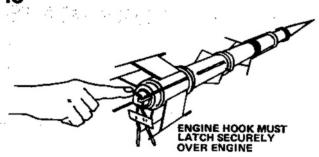
Insert engine into rocket engine mount. Engine hook must latch securely over end of the engine.
