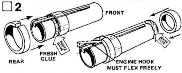
Apply another line of glue around the engine tube just behind the retainer ring. Slide the split adapter ring (part D) onto the rear of the tube and up against the retainer ring. Be sure the notch is centered over the hook, and the hook is straight along the tube. The engine hook must be free to flex slightly as shown. Glue the other adapter ring (part E) to the front of the tube.
