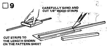
Locate the 1/8" square wood strip (part J) and fine-sand all the sides until smooth. Using the drawing on the pattern sheet labeled 1/8" square strip, lay the wood strip on the drawing and cut to the length shown. Make three identical pieces. Save the left-over wood to be used later.
