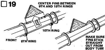
Glue on the three triangular fins, centered between the 9th and 10th rings on the tube. Make sure you use the fin lines between (not same lines as) the three wooden strips at the front of the tube attached in step 10.
