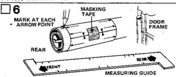
Cut out the body tube marking guide and the measuring guide from the pattern sheet (part I). Wrap the marking guide around the body tube. Match the printed guide marks and tape the guide ends together. Align this joint in the marking guide with the engine hook and mark the tube at each arrow point, front and rear. Draw a straight line connecting each pair of marks. Place the body tube against the inside edge of a door frame as shown. Draw all lines the entire length of the tube.
