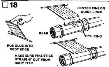
Rub a little glue into the root edge (the edge that attaches to the body) of each of the six large fins. Let the glue set, then apply another line of glue to the fin. Position the fin to the body tube on a fin line as shown. The front end of the fin should be positioned against the number 11 ring as shown. Repeat this procedure for the other five fins. Refer to the illustration to be sure you position the fins correctly.
