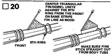
Glue the remaining triangular fin/dowel units against the 8th ring from the front end on the same fin lines as the wood strips. DO NOT set the rocket on its fins while glue is wet. To be sure you positioned all the fins correctly, refer to parts illustration on Page 1.
