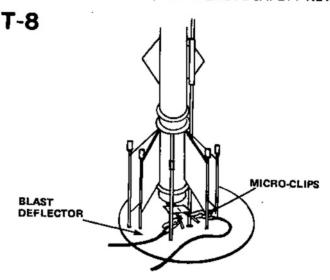
Slide launch rod through rocket launch lug and place rocket on launch pad. Make sure the rocket slides freely on launch rod. Clean the micro-clips and attach them to the igniter wires. Arrange the clips so they do not touch each other or the metal blast deflector. Attach clips as close to engine as possible.
