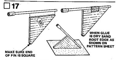
Locate the three triangular fins with the corner missing and glue the remaining three dowels to them as shown on the pattern sheet. When glue is dry, sand root edge of each fin square as shown above
