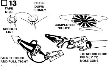
Cut out the parachute (part J) on its edge lines. Cut three equal lengths of shroud line (part K). Attach line ends to the top of the parachute with tape discs (part L) as shown. Form a small loop
