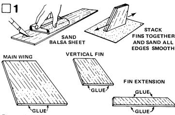
Fine-sand the balsa die-cut sheets (part A). Free the fin edges with a sharp knife, then carefully remove the die-cut fins from the sheets. Stack the fins together into groups as shown and sand all of the edges flat. Lightly sand both sides of each fin. Rub a line of glue into the root edge of each of the fins as shown. Allow the glue to dry completely. Lightly sand the glued edges so that they are smooth.
