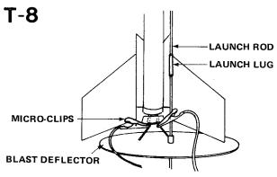
Slide launch rod through rocket launch lug and place rocket on launch pad. Make sure the rocket slides freely on the launch rod. Clean the micro-clips and attach them to the igniter wires. Arrange the clips so they do not touch each other or the metal blast deflector. Attach clips as close to protective tape on igniter as possible.
