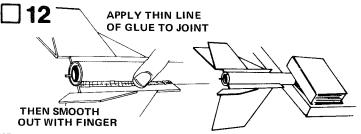
When the glue on the fin joints has dried, apply a glue reinforcement to each fin/body tube joint. Holding the model level, apply a line of glue to both sides of each fin joint. Smooth out the glue with your finger. IMPORTANT - Support rocket on table edge as shown until the glue dries.
