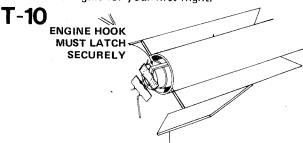
Insert engine into rocket engine mount. Engine hook must latch securely over end of the engine.
