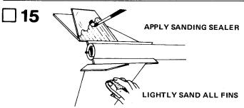
Proper application of sanding sealer makes the rocket look better and reduces drag so that the rocket will fly higher. However, this step is not essential to make a safe, attractive rocket. Apply a coat of sanding sealer to each fin. When sealer is dry, lightly sand all the sealed surfaces. Repeat sealing and sanding process until balsa grain is filled and smooth.
