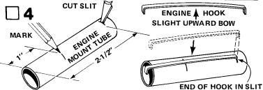
Mark the engine mount tube (part C) at 1" and 2-1/2" from one end. Cut a 1/8" long slit at the 2-1/2" mark. Gently bend the engine hook (part D) so that it bows upward very slightly in the
