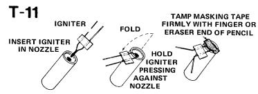
Select an engine and install an igniter as directed in the engine instructions. The engines recommended for use with this rocket are the A8-3, B4-4, B6-4, B8-5, C5-3, and C6-5 made by Estes. Use an A8-3 engine for your first flight.
