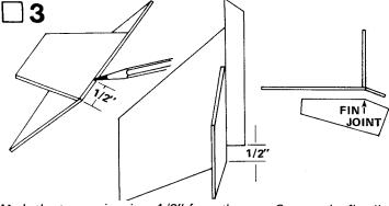
Mark the two main wings 1/2" from the rear. Cut out the fin alignment guide from the pattern sheet (part B). Glue the fin extensions to the main wings so that the longest side is against the main wing and the rear edge is at the mark. Use the guide (part B) to position the wing extensions at the proper angle. NOTE: Check the angle of the wings several times while the glue is drying so that the glue will not set with the wings at the wrong angle.
