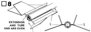
Glue the wing assemblies to the body tube on the alignment lines so that the rear of the wing extensions are even with the rear of the body tube. Adjust the units so that they project straight away from the body tube as shown. Do not set the rocket on its fins while the glue is wet.
