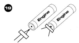
Select an engine for your first launch. This kit uses the following types of engines: A8-3, B4-4, B6-4, B6-6, C6-5 or C6-7. For your first flight use a A8-3 engine. This will give you an approximate altitude of 350 feet (90 m). Carefully insert igniter into engine and bend igniter. Use an engine plug or masking tape to secure igniter in place. Insert engine into rocket until engine clip locks in place, making sure the igniter leads are not touching the engine clip.
