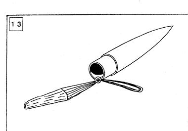
Thread the shroud line loops through the screw eye.
