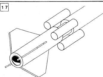
Apply sanding sealer to all four fins. Sand the sealer and apply 3 more coats, sanding between each coat. This step will fill the balsa grain and make your model look better.
