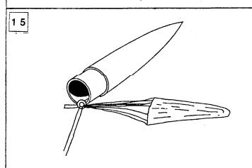
Tie the end of the shock cord through the screw eye.
