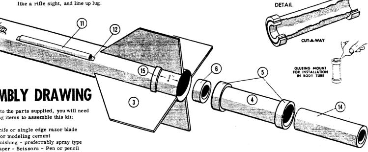
Apply white glue or modeling coment to each fin root chord edge, one at a time, and also along the body tube where fins are to be attached. When glue has just begun to set, place fins in position along the body tube. Stand tube on top end and allow to dry. With the Fin Allignment Guide, check the angle between fins before glue has completely set. Opposite fins should be in line with each other, and adjacent fins should be exactly 90 degrees apart.
