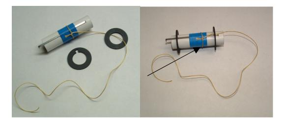
Coat the Kevlar cord where it wraps around the motor mount liberally with glue. Remember, this acts as the anchor point for your recovery system You can set this assembly aside to dry. Now would be a good time to grab a soda!
