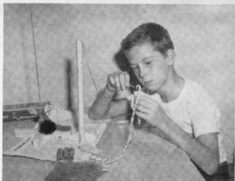
FINS ARE CEMENTED to rocket body, as is launching lug and long rubber band that acts as shock absorber for ejected parachute. Launching stand is assembled, deflection plate nailed to it, parachute tied to rubber band.
