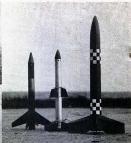
Young contestant at Krakow with typical Polish rockets and launching cradle. Close-up shows winning model at right which attained altitude of 1,817 feet. Body is rolled laminated paper tube, 1.3mm thick with tail end reinforced with 1.5mm plywood to which four plywood fins are attached. Rocket motor body was also of rolled and glued paper with a metal diffuser. Overall length, 13 inches; body diameter 1.12 inches; total fin area 48 sq. in. Meets are run by Polish aeroclub; half the entrants are under 12.
