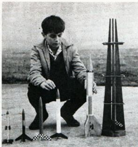
Young contestant at Krakow with typical Polish rockets and launching cradle. Close-up shows winning model at right which attained altitude of 1,817 feet. Body is rolled laminated paper tube, 1.3mm thick with tail end reinforced with 1.5mm plywood to which four plywood fins are attached. Rocket motor body was also of rolled and glued paper with a metal diffuser. Overall length, 13 inches; body diameter 1.12 inches; total fin area 48 sq. in. Meets are run by Polish aeroclub; half the entrants are under 12.
