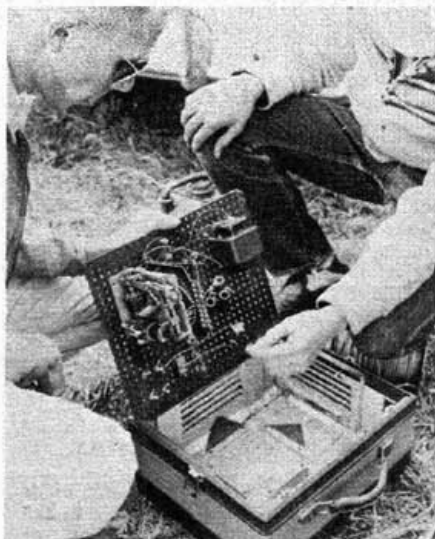
Lynn Ericson demonstrates his electronic firing panel which goes through automatic checkout and count-down procedure for launching model rockets.
