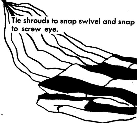
Tie shrouds to snap swivel and snap to screw eye.
