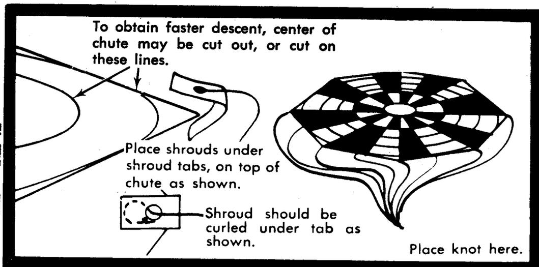
To obtain faster descent, center of chute may be cut out, or cut on these lines.
