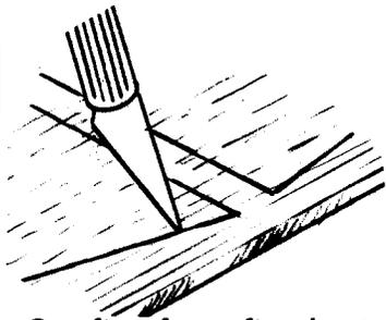
Cut fins from fin sheet. If possible use a ruler to help you get a good straight edge. Large fins are for the booster and small fins for the body tube.
