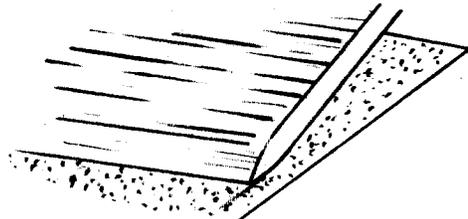
Sand the three edges of fins that do not attach to body tube. Sand the fin surfaces smooth.
