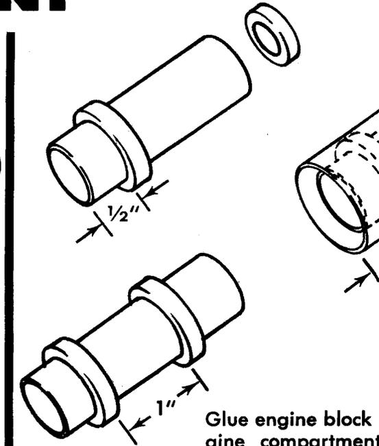
Glue engine block engine compartment centering ring 1/2" from the end of the tube. Glue the other ring. Glue unit inside that bottom ring is flush with the end of the tube.
