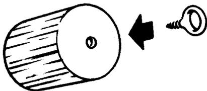
Put the screw eye into the coupler then remove it. Then put glue in the hole and replace the screw eye.
