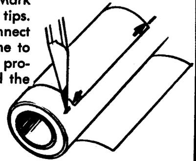
For best adhesion of paint and glue, sand tubes until all gloss is removed.
