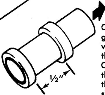
Glue one centering ring on the engine compartment so that it is flush with one end. Glue the other ring so that it is 1/2" from the first ring. Glue this unit in the booster tube so that the bottom ring is flush with the end of the tube. The top ring should fit against the joiner.
