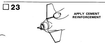
After all cement has dried, give each fin and rudder joint a plastic cement reinforcement. Hold model level and apply a line of tube-type plastic cement to both sides of each fin joint. Rub cement into missile body/fin joint and smooth out the cement with your finger. Keep the model level until cement dries.
