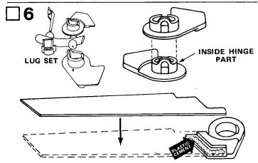
Remove the wing hinge halves from the plastic hinge/lug set (part G). Carefully sand the hinge part that goes inside the other that until the assembled parts rotate easily, but do not sand so much to cause them to be too loose. Pull the two pieces apart and cement a wing hinge half to each wing with tube-type plastic cement, making sure the wing fits correctly into the area provided in the wing hinge half as shown. Allow these parts to dry thoroughly.
