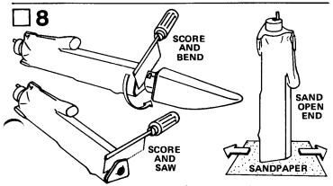
Lightly score around the nose cone/body joint with a razor saw on the Cruise Missile body (part H). Bend body gently so it breaks apart at the scored line. Using the razor saw cut the missile body along the edge of the shoulder and missile body as shown. Lay a sheet of sandpaper flat on your work surface and pass the open end of the body across it to smooth out the edges. Be careful not to sand off too much of the plastic.
