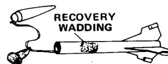
Loosely pack three or four squares of flameproof wadding into the body tube from the shock cord end. Fold the streamer in half lengthwise from where it is attached to the shock cord. Roll the streamer compactly enough to enter the body tube easily. Push the rolled streamer down into the body tube on top of the wadding.
