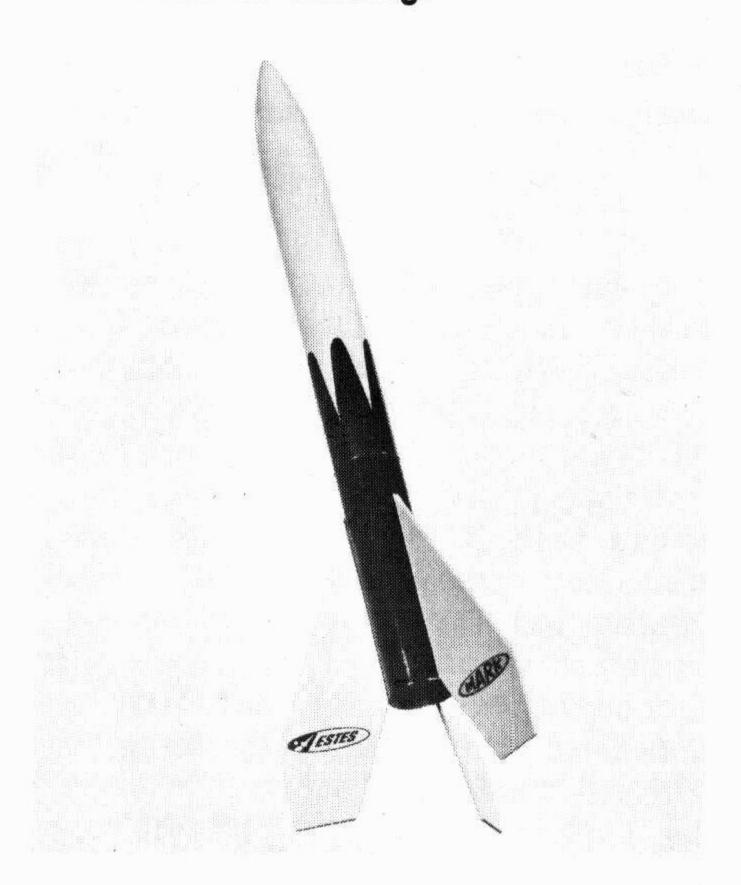
The streamer-recovery Mark II was designed by Larry Renger, who chose a spiral-wound tube that is lighter and truer in shape than the type used on the older Mark.
