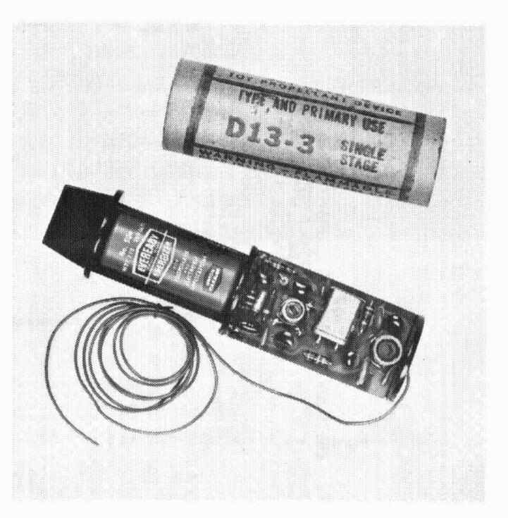
Our "Transroc" opens up a whole new world for the rocketeer. It fits neatly into a BT-50 and transmits over distances of more than 1/2 mile. Battery life in the beacon mode is over 24 hours. The Transroc uses a trailing wire antenna and
